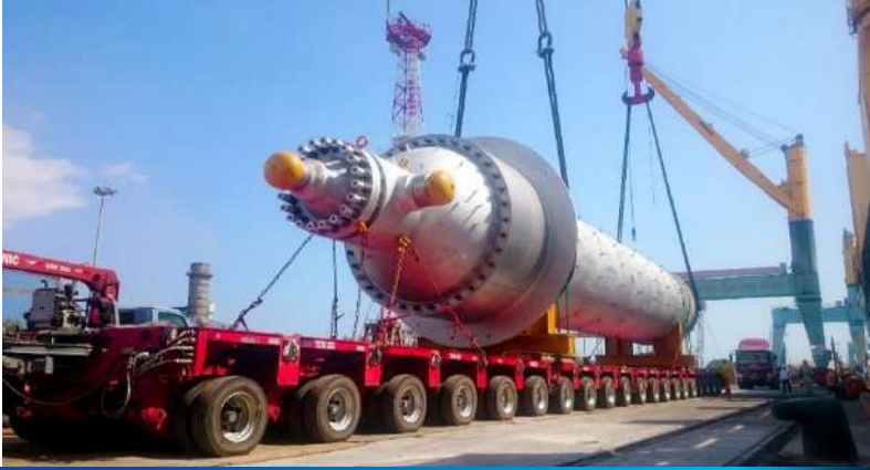
26 Axle Lines Hydraulic Modular Trailer includes: 3 units of 6 axles and 2 units of 4 axle
