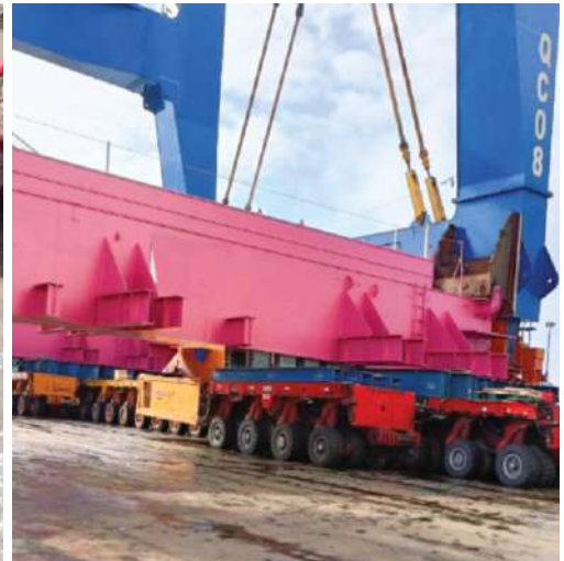
44 Axle Lines Hydraulic Modular Trailer include 6 units of 6 axles and 2 units of 4 axles Loading capacity 1,304 tons
