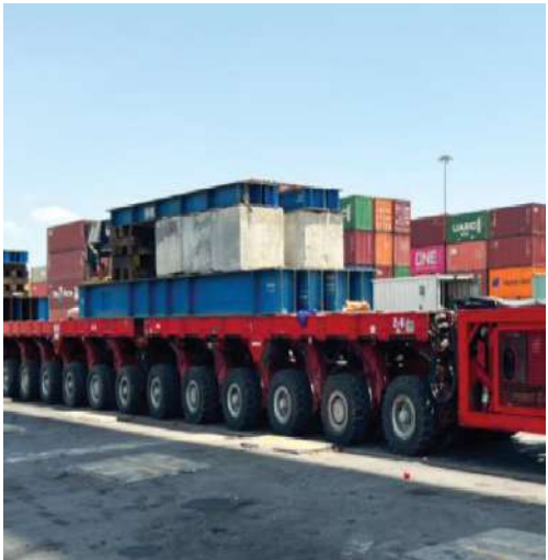
44 Axle Lines Hydraulic Modular Trailer include 6 units of 6 axles and 2 units of 4 axles Loading capacity 1,304 tons
